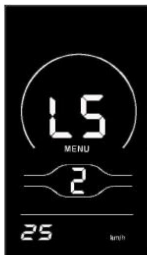
Speed limit setting interface
