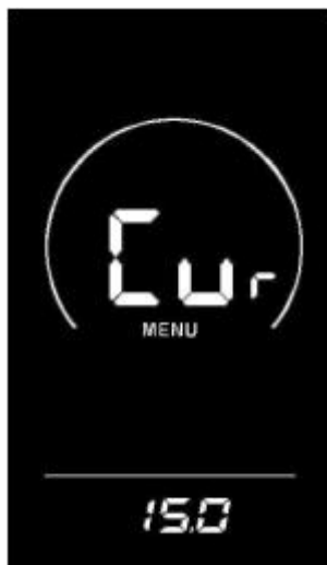
Current limit value setting interface
