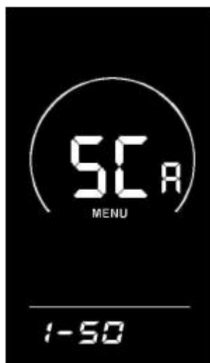
PAS ratio value setting interface
