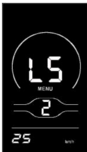
Speed limit setting interface
