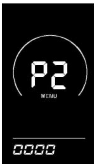
Power-on password input setting interface
