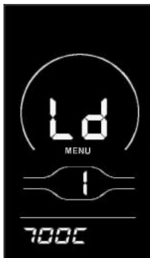
Wheel diameter setting interface
