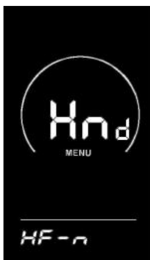
Throttle gear enable setting interface
