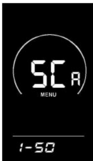
PAS ratio value setting interface
