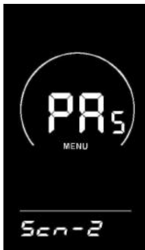
Booster sensor sensitivity setting interface
