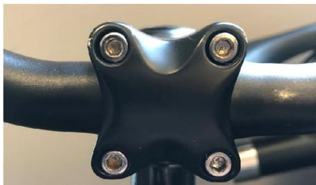
**Step 3:** Align your handlebars using your 5mm hex wrench. Loosen the two stem bolts using your 5mm hex wrench and align the handlebars to be perpendicular to the bike frame. Tighten top bolt first, then the two stem bolts to hold the handlebar position in place.
