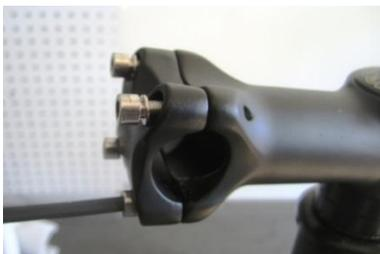
Install the handlebar and re install the clamp to fit the handlebar in place.
