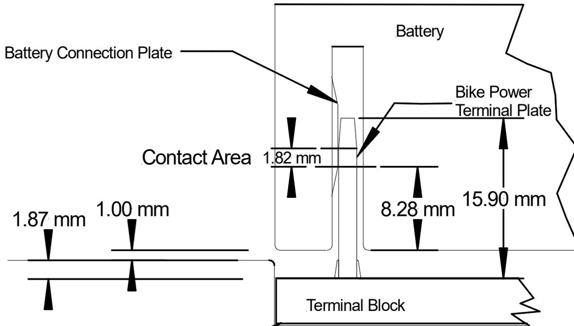
Terminal block can be spaced up 2mm to improve electrical contact area from 1.8mm to 3.8mm
