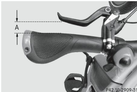
Before every ride, carry out a stationary brake test. To do so, pull the brake levers towards the handlebar using two fingers and normal braking force. The brake lever must not come into contact with the handlebar (▷ page 24). A distance “A” must remain between the brake lever and the handle, even when maximum hand force is applied.
