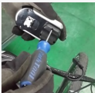
Removal of Display Wiring Harness
