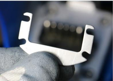
**4** Take the special spacer (2120-WASHER-520) and hold it with the open side up.
