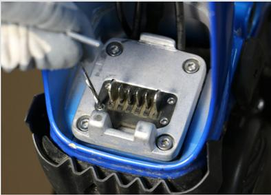
**2** Remove the 4 screws of the battery connector
