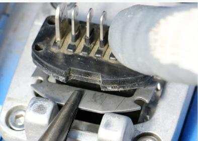
**5** Place the spacer underneath the connector in the recess of the connector bracket. It can be helpful to use needle nose pliers.
