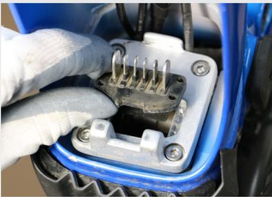
**3** Lift the connector up out of the bracket, as far as it will go without too much force. Avoid pulling too hard on the connector, as this might damage the wires.
