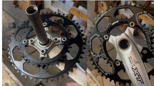
old9 speed XT hollow tech triple setup as a double
