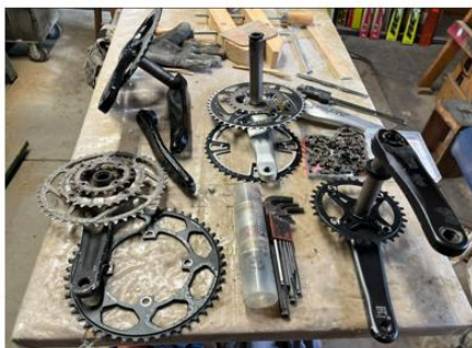
variety of cranksets consider to meet lower gear requirements.
