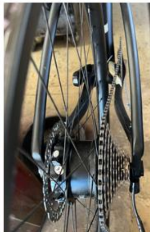
frt large to aft large chain line
