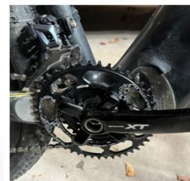
final crankset selection , raceworks XT with 46/28 t, Utrera front derailleur
