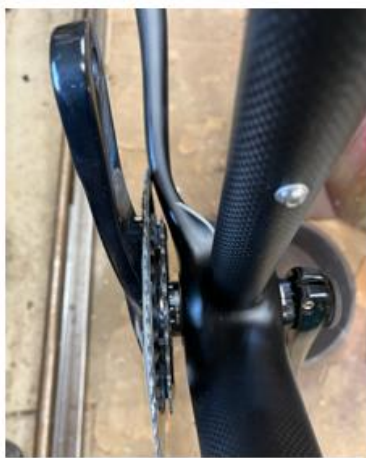
50 tooth chain ring hitting the chain stay
