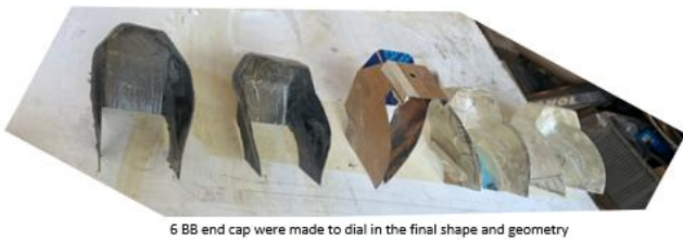
6 BB end cap were made to dial in the final shape and geometry
