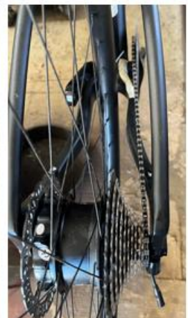
frt small to aft small chain line
