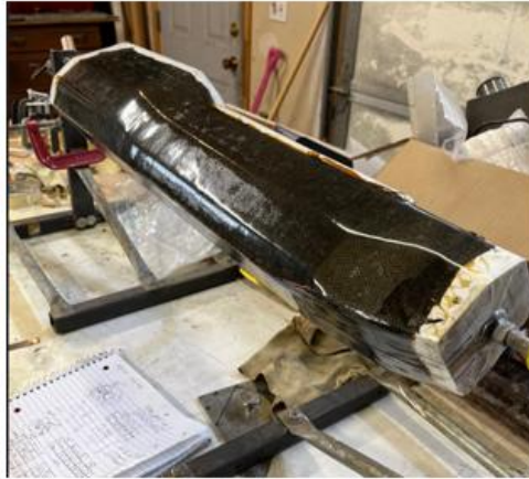
down tube battery shell on wood mandrel
