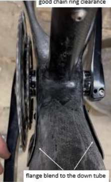
flange blend to the down tube
