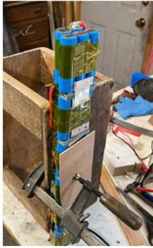
battery pack in vertical positon to connect the bottom to the top
