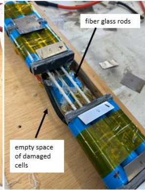
damaged cells from spot weld going through the nickel strip put fiber glass sheets under all the tabs after this happened
