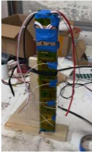
BMS wires on the bottom 3 parallel cells
