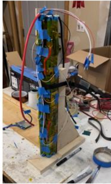
BMS wires on the top cell, & wire routing
