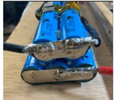
main (+,-) cable connection
