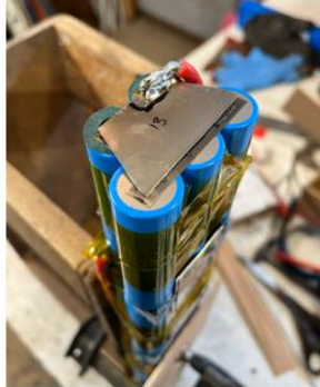
bottom to top serial connection .2 thick nickle tab
