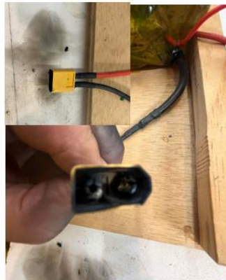
always put the female connector side on the hot side of the circuit
