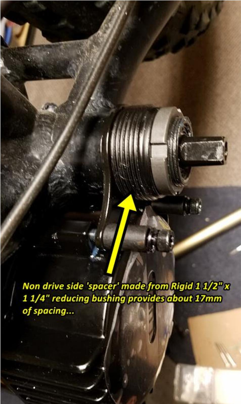
***Non drive side 'spacer' made from Rigid 1 1/2" x 1 1/4" reducing bushing provides about 17mm of spacing...***
