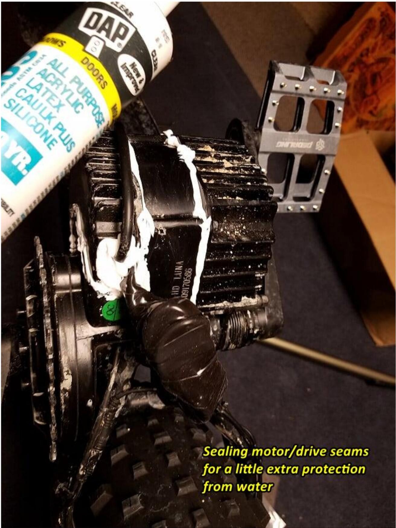
*Sealing motor/drive seams
