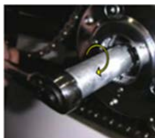
4pin socket for central Syncdrive MY07/MY12 (part# 2520-FY06-03V)
