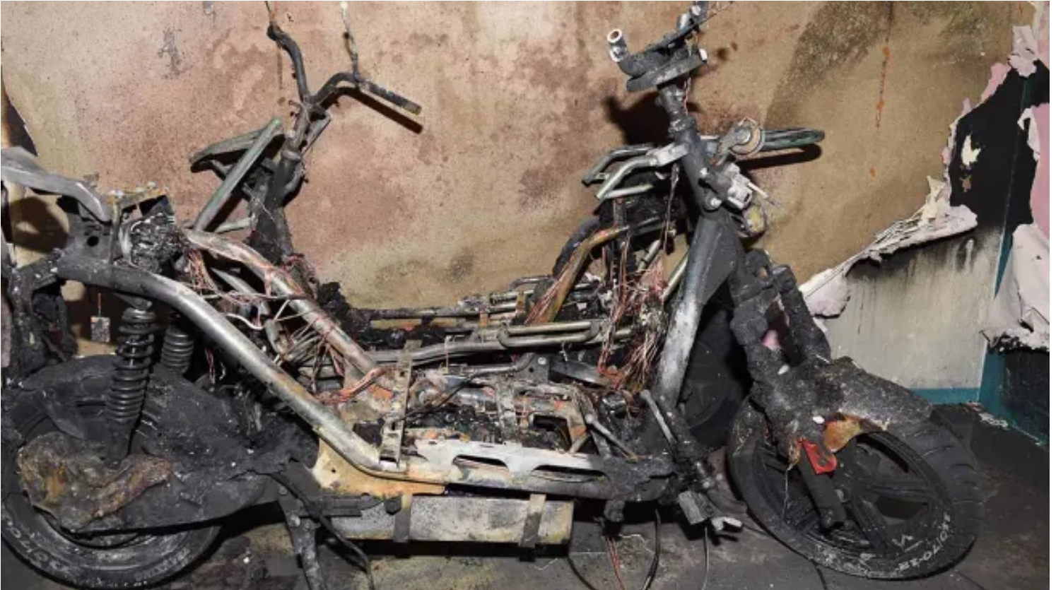
A January 2022 fire in the Bronx borough of New York City was caused by the battery in an electric scooter. Source: FDNY
