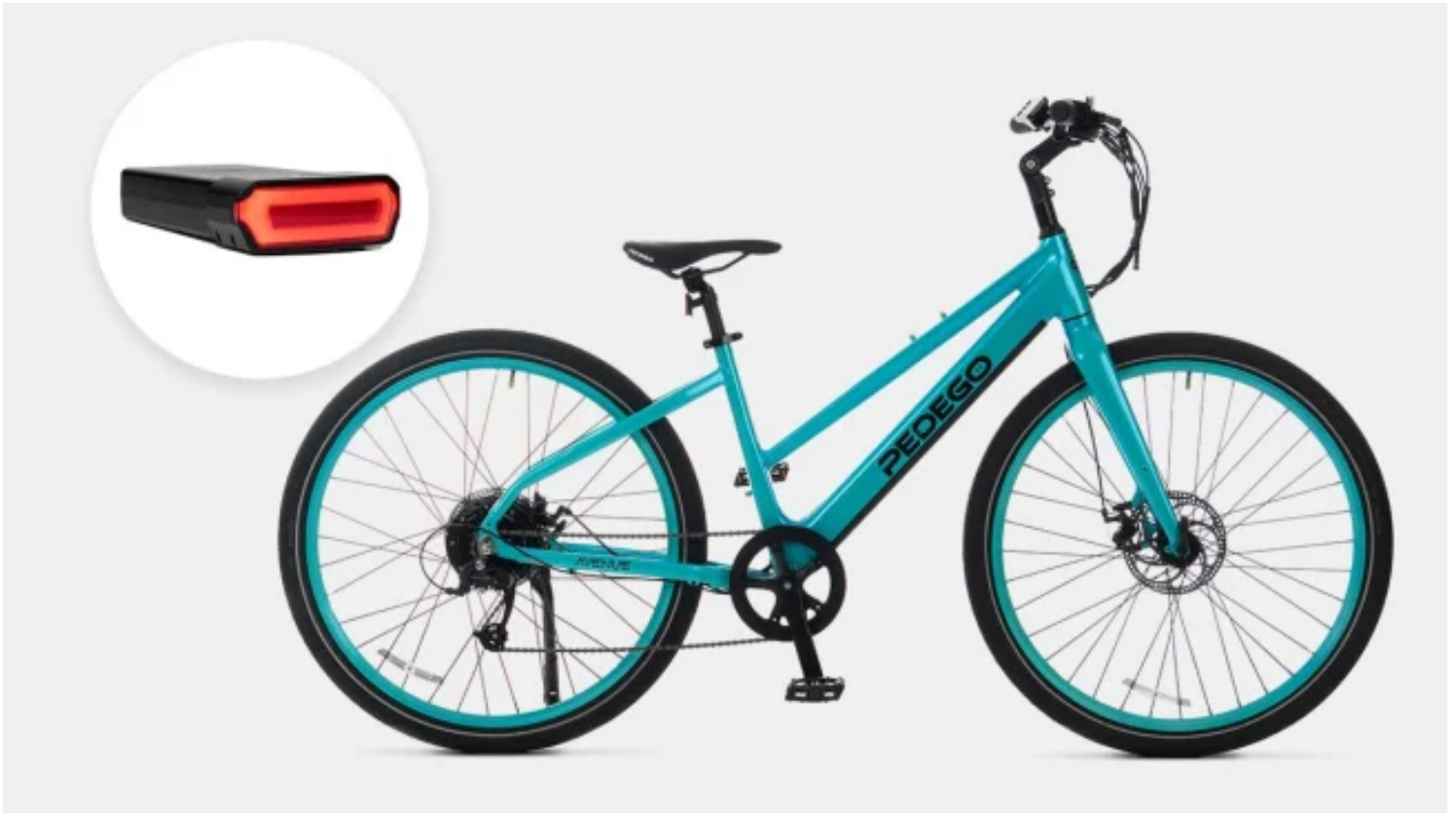
The California e-bike company Pedego switched to a new supplier and battery (inset photo) after it received reports of batteries catching on fire.
