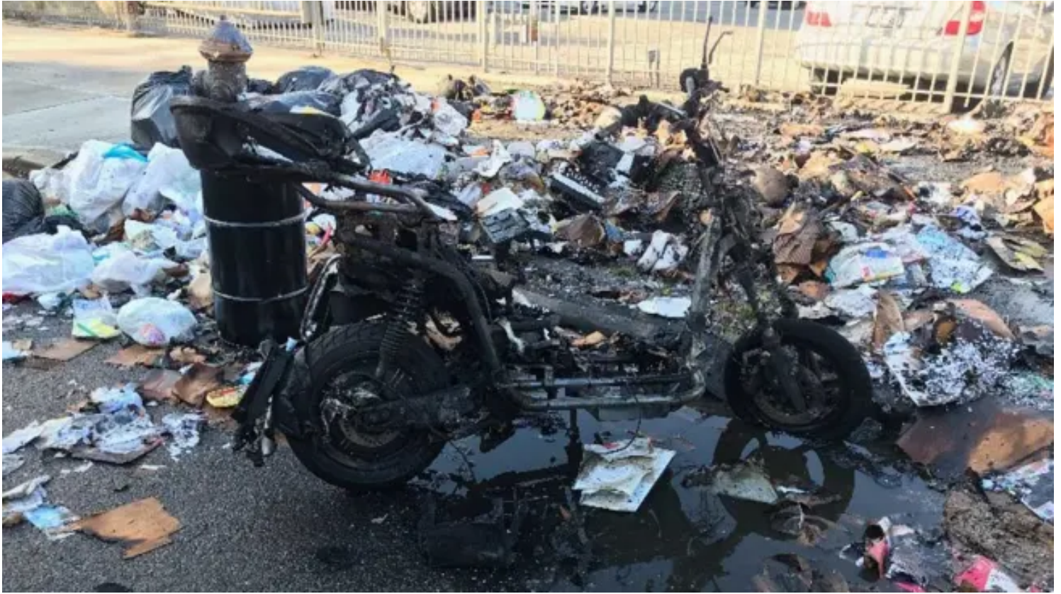
Remnants of an April 2022 fire in New York City triggered by the battery in an electric bike/scooter.
