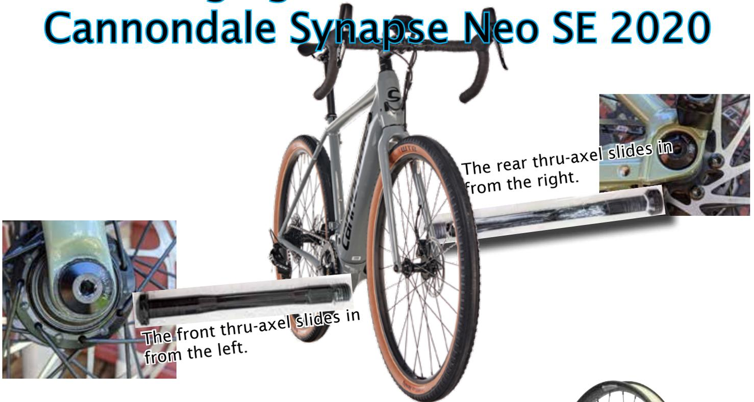
The Synapse comes with two thru-axles; to loosen turn the “Max 11Nm” end counter-clockwise. If the thru-axle was actually tightened to the maximum of 11 Newton Meters (Nm) it may take some effort to get it to loosen.
