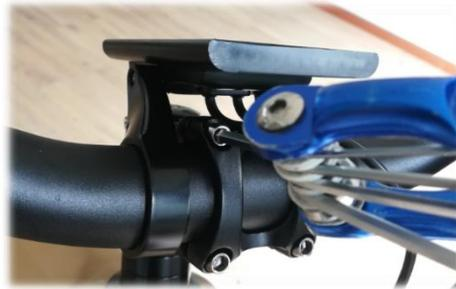
b.Place the handlebar on the stem ,then put the bracket and 4 screws back into place.
