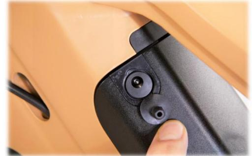
b. To charge the battery, remove the rubber plug from the side of the bike. Plug the charger into the power outlet and wait until the light on the charging unit is illuminated. Plug the other end of the cord into the bike. The light will change to green when it's charged. (2 batteries, two charging ports).
