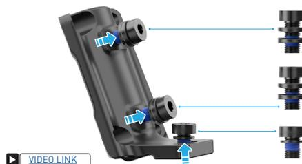
1. The three mounting bolts for the Front Rack will ship pre-assembled into the head plate and must be removed before assembly. Note the position of each bolt and the washers on each bolt. These must be reassembled back in the same position and orientation.
